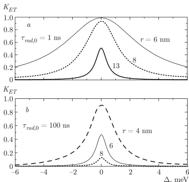
**Fig. 4.** Dependence of the energy transfer efficiency  $K_{ET}$  on the donor–acceptor energy detuning  $\Delta$  for (a)  $\tau_{rad,0} = 1$  ns and (b)  $\tau_{rad,0} = 100$  ns. The thick solid, dotted, thin solid, and dashed curves correspond to the respective donor–acceptor distances  $r = 13$  nm, 8 nm, 6 nm, 4 nm. The other calculation parameters are the same as in Fig. 2
