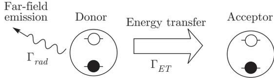
Fig. 1. Schematic illustration of the energy transfer and photon radiation processes
