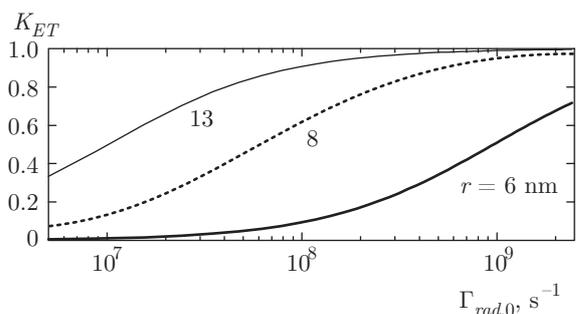
**Fig. 3.** Dependence of the energy transfer efficiency  $K_{ET}$  on the radiative rate  $\Gamma_{rad,0}$  for different donor–acceptor distances  $r$ . The calculation has been performed for  $\Delta = 0$  and the other parameters the same as in Fig. 2
