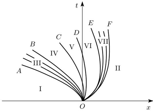
**Fig. 3.** Two magnetogravity rarefaction waves and two Alfvénic waves over a slope. I, II, IV, V, VI are regions of uniformly accelerated flow; III and VII are magnetogravity rarefaction waves;  $OC$  and  $OD$  are Alfvénic waves
