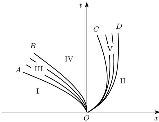
**Fig. 6.** Two hydrodynamic rarefaction waves and a vacuum region between them over a slope. I and II are regions of uniformly accelerated flow; III and V are magnetogravity rarefaction waves; IV is the vacuum region
