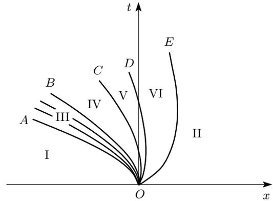
**Fig. 4.** Magnetogravity shock wave, magnetogravity rarefaction wave, and two Alfvénic waves over a slope. I, II, IV, V, VI are regions of uniformly accelerated flow; III is a magnetogravity rarefaction wave;  $OC$  and  $OD$  are Alfvénic waves;  $OE$  is a magnetogravity shock wave
