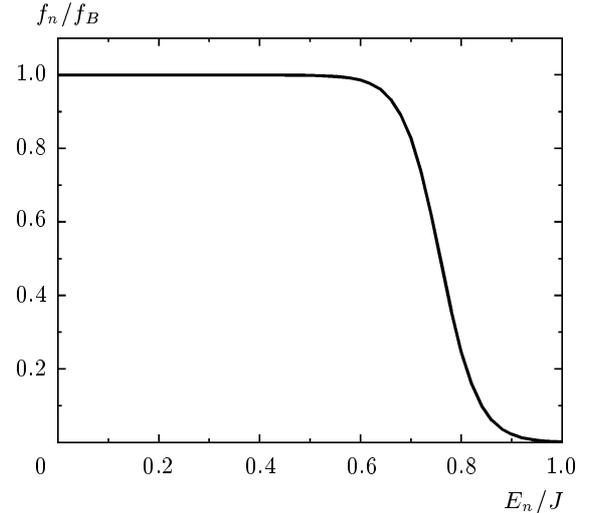
**Fig. 6.** Relation of the distribution function  $f_n$  for population of highly excited electron states of atoms to the Boltzmann distribution function  $f_B$  in the course of stepwise ionization or three-body electron-ion recombination
