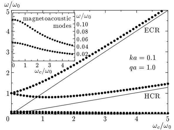
**Fig. 4.** The dipole crystal collective excitations as a function of the magnetic field. ECR and HCR are the electron and hole cyclotron energies in the GaAs/AlGaAs structure. The inset shows the magnetoacoustic modes in enlarged scale
