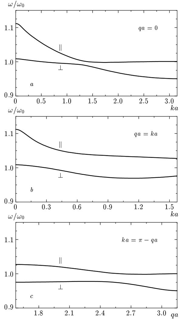
**Fig. 2.** Dispersion of the optical longitudinal and transverse modes: (a)  $\Gamma$ - $L$  direction, (b)  $\Gamma$ - $X$ , and (c)  $L$ - $X$
