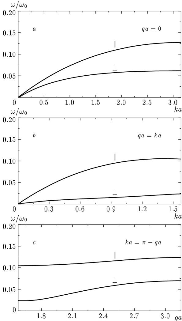
**Fig. 3.** Dispersion of the acoustical longitudinal and transverse modes: (a)  $\Gamma$ -L direction, (b)  $\Gamma$ -X, and (c) L-X
