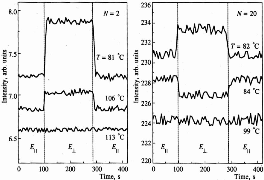
**Fig. 1.** Optical reflection intensity for thin ( $N = 2$ ) and thick ( $N = 20$ ) ferroelectric films in an electric field applied parallel ( $E_{\parallel}$ ) and perpendicular ( $E_{\perp}$ ) to the direction of polarization of the light ( $\lambda = 600$  nm). For thick film ( $N = 20$ ), the change in reflection intensity when the direction of the electric field is changed is different at low ( $T = 82^{\circ}\text{C}$ ) and high ( $T = 84^{\circ}\text{C}$ ) temperatures (8SI\*)
