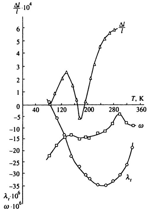
FIG. 2. Anisotropic  $\lambda$ , and volume  $\omega$  magnetostrictions versus temperature measured at  $H=10$  kOe and relative thermal expansion  $\Delta l/l$ .
