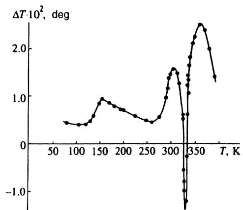
FIG. 3. Amplitude of the magnetocaloric ( $\Delta T$ ) effect versus temperature recorded at  $H=11$  kOe.
