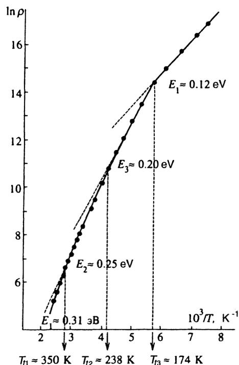
FIG. 5. Logarithm of sample resistivity as a function of  $1/T$ .
