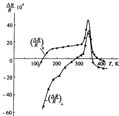
FIG. 4. Transverse  $(\Delta R/R)_{\parallel}$  and longitudinal  $(\Delta R/R)_{\perp}$  relative magnetoresistances as functions of temperature measured at  $H = 10$  kOe.
