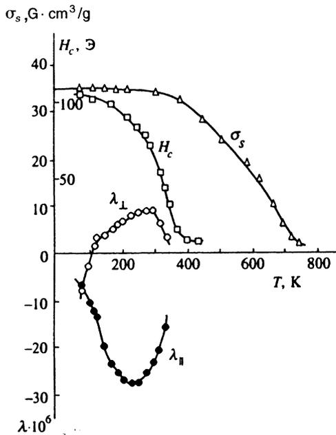
FIG. 1. Spontaneous magnetization  $\sigma_s$ , coercive force  $H_c$ , perpendicular  $\lambda_{\perp}$  and parallel  $\lambda_{\parallel}$  magnetostrictions as functions of temperature measured under a magnetic field  $H=10$  kOe.
