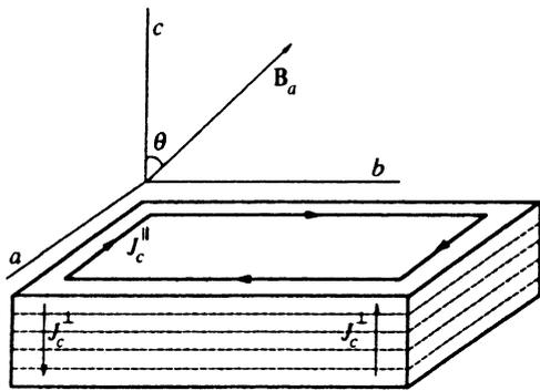
FIG. 1. Orientation of the single crystal relative to the field.
