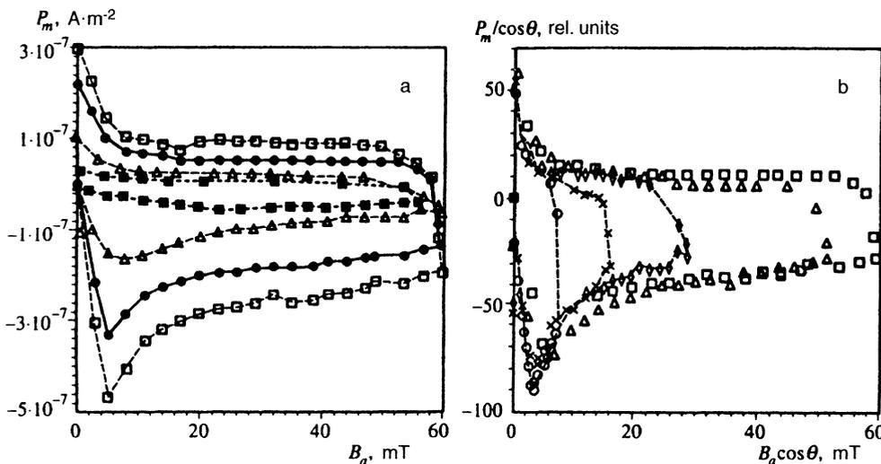
FIG. 3. Hysteresis curves for several values of  $\theta$ : a— $\theta=0^\circ$  ( $\square$ ),  $45^\circ$  ( $\bullet$ ),  $61^\circ$  ( $\triangle$ ),  $82^\circ$  ( $\blacksquare$ ); b —  $\theta=0^\circ$  ( $\square$ ),  $30^\circ$  ( $\triangle$ ),  $61^\circ$  ( $\diamond$ ),  $74^\circ$  ( $\times$ ),  $82^\circ$  ( $\circ$ ).
