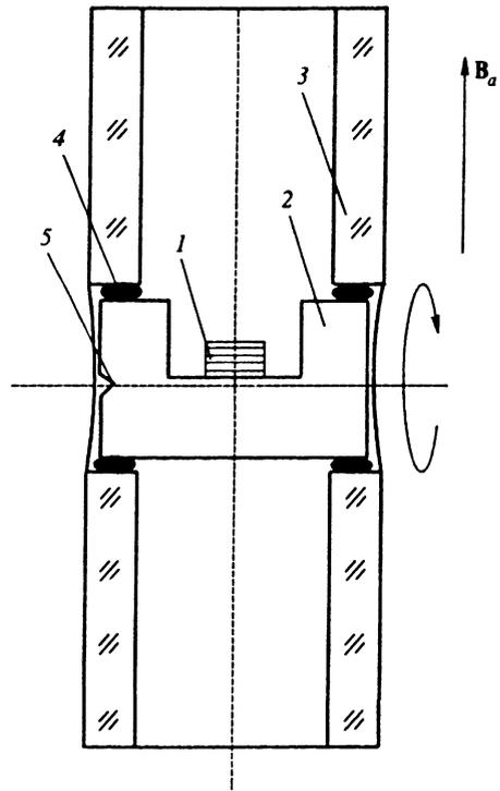
FIG. 2. Quartz holder: 1 — single crystal, 2 — movable quartz cylinder, 3 — quartz tube, 4 — Ramsay cylinder, 5 — ruled line on the end surface of the flat cylinder.
