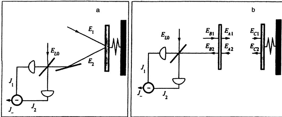
FIG. 1. (a) Simple and (b) interferometric optical displacement sensors. A change in the mobile mirror position due to the detected force leads to a phase shift in the reflected wave, which is measured by a balanced homodyne circuit.
