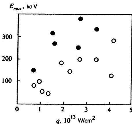
FIG. 2. Dependence of the maximum energy of the high-energy electrons on the flux density of the laser radiation on the target for an aluminum plasma heated by a nanosecond laser pulse; the open circles and black circles are for  $p_1 = 10^{-2}$  torr and  $p_2 = 10^{-5}$  torr, respectively.
