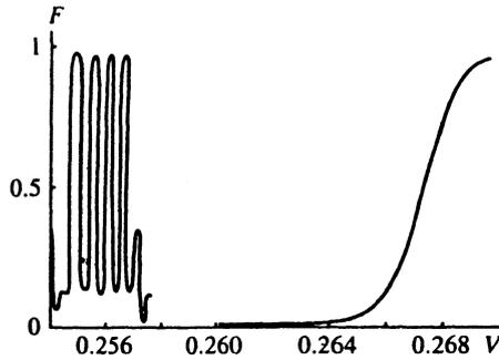
FIG. 4. Energy flux through the plane  $x_f=10$  plane during the time  $\Delta t_f=200$  for a  $K\bar{K}$  system as a function of the initial kink velocity  $V$ . The region near the resonance limit point at  $V_{cr}\approx 0.2598$  is shown (since the resonant "windows" are extremely narrow, they have been partially omitted).
