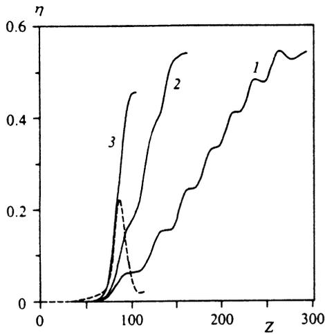
FIG. 2. Dependence of the efficiency  $\eta$  of a free-electron laser on the dimensionless length  $Z$ : 1)  $\xi=0.01$ , 2)  $\xi=0.04$ , 3)  $\xi=0.07$ . The initial amplitude of the electromagnetic wave is  $\alpha_s(0)=0.02$ .
