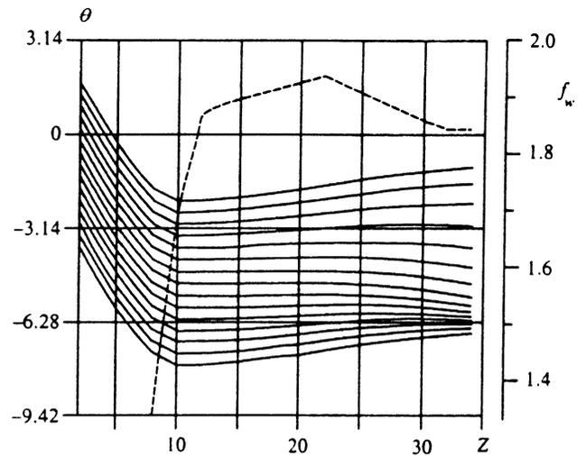
FIG. 1. Dependence of the normalized wiggler field  $f_w$  in the buncher segment (dashed line; the nominal value  $f_w = 1.88$ ) and of the phases of the electrons  $\theta$  (solid lines) on the dimensionless length  $Z$ . The initial amplitude of the electromagnetic wave  $\alpha_s(0) = 0.02$ .
