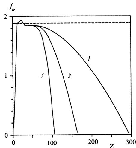
FIG. 3. Dependence of the normalized wiggler field  $f_w$  on the dimensionless length  $Z$ : 1)  $\xi=0.01$ , 2)  $\xi=0.04$ , 3)  $\xi=0.07$ . The dashed line corresponds to the nominal value of  $f_w$ .
