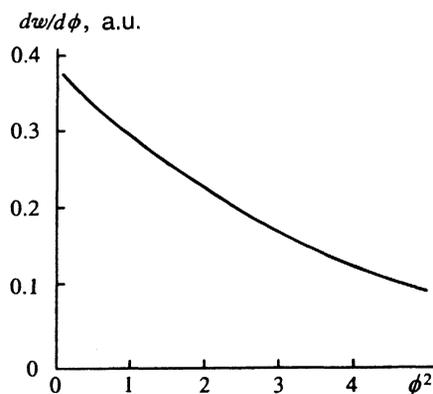
FIG. 2. Angular distribution of photoelectrons as a function of  $\phi = \psi/\omega$  for field strength  $F=0.3$  a.u.
