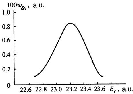
FIG. 3. Energy spectrum of the outgoing photoelectrons for ionization by a circularly polarized radiation field with amplitude  $F=0.3$  a.u. and frequency  $\omega=1.2$  eV $\approx 0.044$  a.u. as a function of the photoelectron kinetic energy  $E_e$ .
