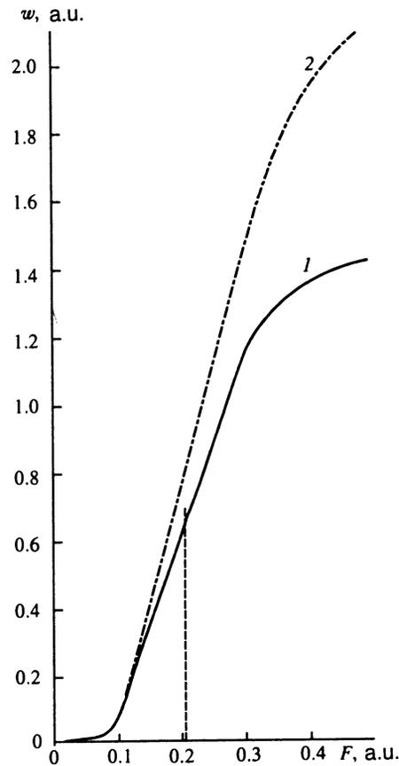
FIG. 4. Ionization probability per unit time due to a strong low-frequency field from the ground state of a hydrogen atom: 1) calculated from Eq. (25) for barrier-suppression ionization; 2) calculated from Eq. (17) for tunneling ionization. The broken vertical line corresponds to the field strength  $F_{\text{BSI}}$  for which the energy level equals the peak of the effective potential barrier, i.e., for which above-threshold decay of the atom is possible classically.
