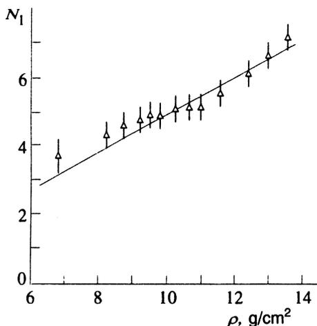
FIG. 2. Coordination number of extended liquid mercury along the saturation line (Ref. 13).
