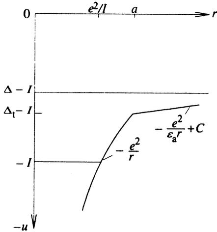
FIG. 1. Screened ion potential. Hatching indicates the conduction band bottom.
