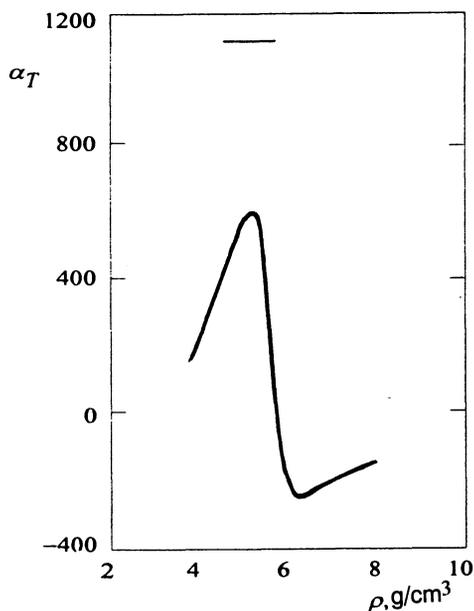
FIG. 5. Thermoelectric power of mercury for  $T=1773$  K. The curve: experiment (Ref. 14) Hatching indicates the upper estimate corresponding to the hole conduction.
