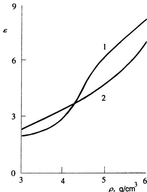
FIG. 3. Permittivity of mercury vapor versus density for  $T = 1773 \text{ K}$ . 1—experiment (Ref. 3). 2—regularized third-order Clausius-Mosotti equation.
