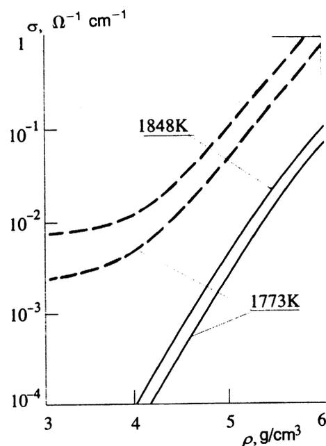
FIG. 4. Mercury vapor conductivity versus density for various temperatures. Dashed lines: experiment (Ref. 3); solid lines: theoretical estimate.
