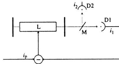
FIG. 1. Optical layout used in Ref. 12. L—laser; D1 and D2—detectors; M—beamsplitting mirror. The photocurrent from detector D2 modulates the laser pump current  $i_p$  via the feedback loop.
