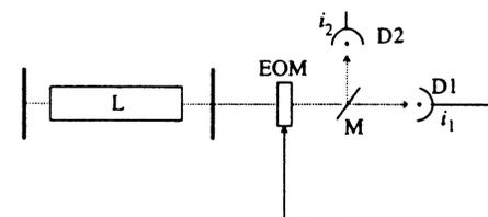
FIG. 2. Optical layout used in Ref. 14. Notation as in Fig. 1. Feedback is implemented via the electrooptic modulator (EOM).
