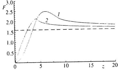
FIG. 1. Function  $F$  (volt-ampere characteristic) for a tunneling junction made of two identical superconductors, for bilateral (curve 1) and unilateral (curve 2) coating of the dielectric by a normal metal layer of thickness  $d$ . Dash-dot horizontal line is the asymptote ( $\pi/2$ ) of the function  $F$  for  $Z \rightarrow \infty$ .
