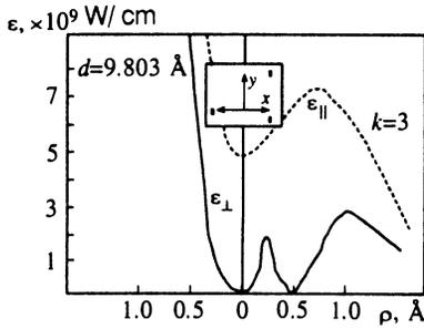
FIG. 1. Electric field components in the Møller approximation for the atomic potential for the  $\langle 111 \rangle$  channel in a Ge crystal as a function of the distance  $\rho$  from the center of the channel;  $k$  is the index of the Fourier harmonic.
