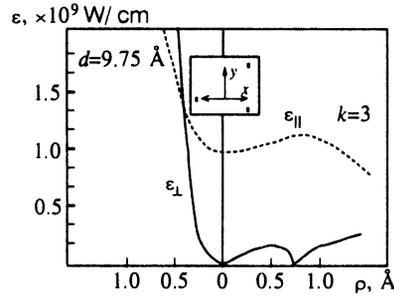
FIG. 2. Electric field components in the Møller approximation for the atomic potential for the  $\langle 111 \rangle$  channel in a NaCl crystal as a function of the distance from the center of the channel;  $k$  is the index of the Fourier harmonic.
