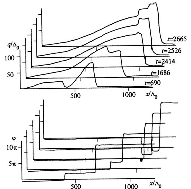
FIG. 9. Numerical solution of the Slonczewski equations for two VBL with charges  $N_1=4$  and  $N_2=16$ , for  $v=0.5972$  and  $H_x=0.157$ . Upon collision, an infinite generation of  $2\pi$  VBL pairs sets in.
