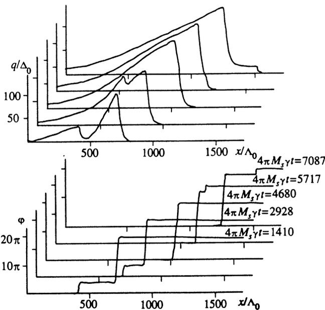
FIG. 7. Numerical solution of the Slonczewski equations at different times for two VBL with the charges  $N_1=4$  and  $N_2=16$ , for  $H_x=0.0314$ ,  $v=0.25$ , and  $b^2=10^{-4}$ .
