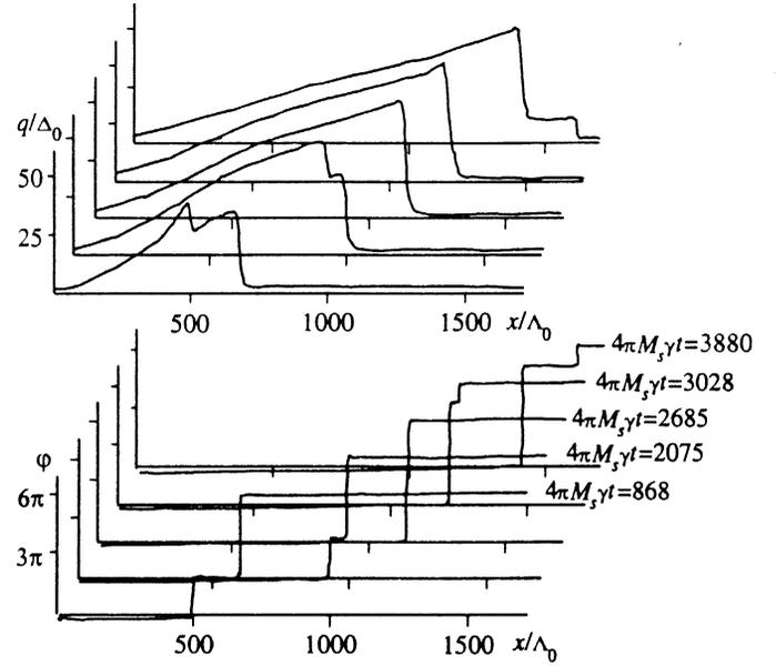
FIG. 5. Numerical solution of the Slonczewski equations at different times for two VBL with charges  $N_1=2$  and  $N_2=4$ , for  $H_x=0$ ,  $b^2=10^{-4}$  and  $v=0.4567$ .
