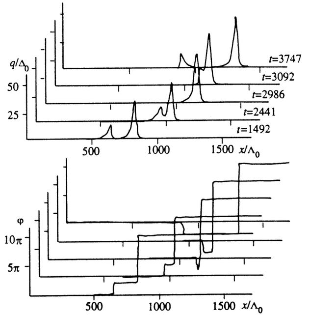
FIG. 8. Numerical solution of the Slonczewski equations for two VBL with charges  $N_1=2$  and  $N_2=8$ ,  $v=0.3683$ ,  $H_x=0.157$ , and  $b^2=5 \cdot 10^{-3}$ . Upon collision, the  $2\pi$  VBL coming up from behind is reflected.
