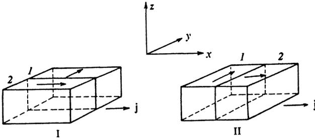
FIG. 1. Connection of the resistances of the domains. I—Parallel connection; II—series connection. The arrows show the directions of the antiferromagnetism vectors  $\mathbf{L}$  in domains 1 and 2.
