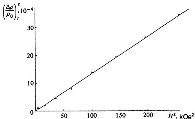
FIG. 3. Transverse magnetoresistance  $(\Delta\rho/\rho_0)_t^2$  versus the square of the magnetic field for the orientation  $\mathbf{H} \parallel [001]$  at  $T = 106$  K in  $\text{FeGe}_2$ .
