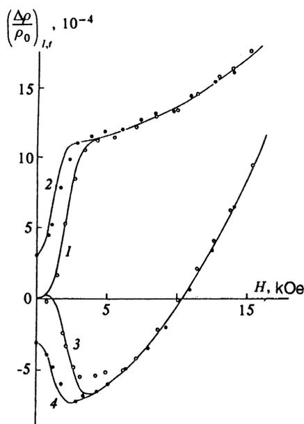
FIG. 4. The longitudinal magnetoresistance  $(\Delta\rho/\rho_0)_l$  (curves 1 and 2) and the transverse magnetoresistance in the antiferromagnetism plane  $(\Delta\rho/\rho_0)_t$  (curves 3 and 4) versus  $H$  at  $T = 106$  K in  $\text{FeGe}_2$ . 1, 3—Virgin magnetization curve; 2, 4—descending branch of the hysteresis loop. Solid curves Calculated from (28); open and filled circles) experimental.
