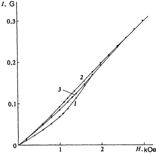
FIG. 2. The specific magnetization  $I_\alpha$  of an FeGe<sub>2</sub> single crystal versus the magnetic field  $H$  for the case  $\mathbf{H} \parallel [110]$  at  $T=106$  K. 1—Virgin magnetization curve; 2, 3—hysteresis loop.
