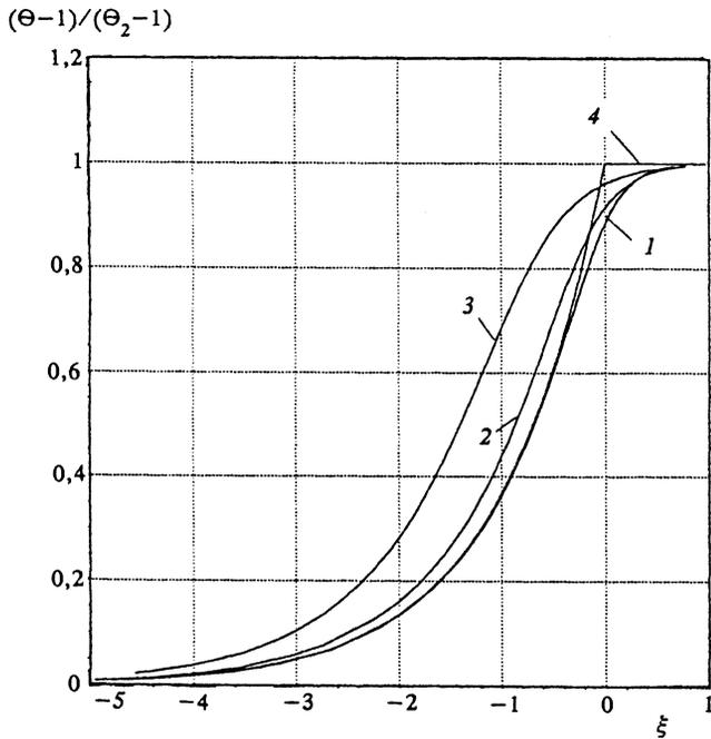
FIG. 1. Scaled temperature profiles in a combustion wave: 1)  $\mathcal{E}=70$ ,  $\Theta_2=8$ ,  $\ln \Lambda=14.3$ ; 2)  $\mathcal{E}=42$ ,  $\Theta_2=6$ ,  $\ln \Lambda=11.7$ ; 3)  $\mathcal{E}=21$ ,  $\Theta_2=3$ ,  $\ln \Lambda=10.4$ ; trace 4 corresponds to Eq. (12).
