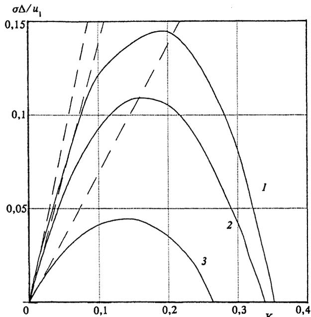
FIG. 2. Instability growth rate  $\sigma\Delta/u_{z1} = SK$  versus the dimensionless wave number  $K = k\Delta$ . The numbers labeling the traces correspond to the temperature profiles in the combustion waves shown in Fig. 1. The dashed straight lines correspond to solutions in the model of a discontinuous flame front.
