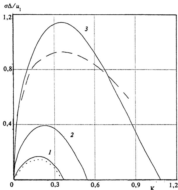
FIG. 3. Dimensionless growth rate as a function of wave number for a flame propagating in a gravitational field with different values of the Froude number: 1)  $Fr=10$ ; 2)  $Fr=1$ ; 3)  $Fr=0.1$  for  $\Theta_2=\delta$ . The dots correspond to the case of zero gravitational field and the dashed curve corresponds to the analytical result (65).
