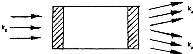
FIG. 1. Scheme for observing Ramsey interference in parametric light scattering: the pump photon  $k_0$  decays into two photons  $k_a$  and  $k_b$  as a result of coherent mixing in the two nonlinear crystals (hatched regions) separated by a linear medium, in particular, air.
