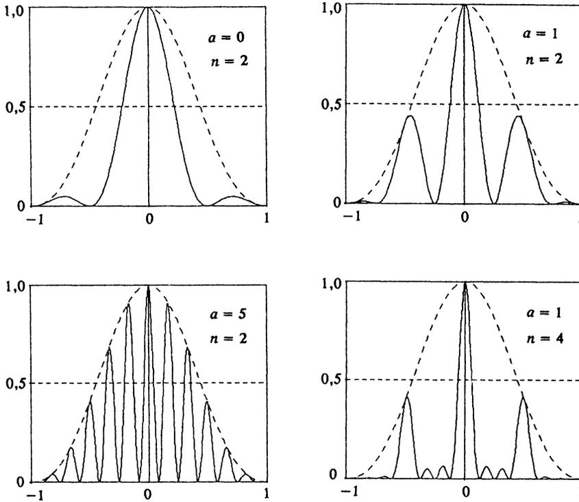
FIG. 2. Spectrum of parametric scattering by  $n$  sequentially arranged crystals. Dimensionless frequency  $(\omega - \omega_0)\tau/2\pi$  is plotted along the abscissa, the parameter  $a = \tau/\tau'$  is proportional to the ratio  $l'/l$  of the length of the gap between the crystals to their length. The dashed curve (the envelope of the spectrum) is the spectrum for the case of dispersion cancellation, i.e., for  $a = -1$ .
