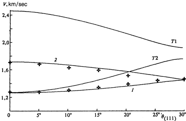
FIG. 5. Velocity of surface and volume acoustic waves for the (111) plane of a PbTe crystal as a function of the angle  $\theta_{(111)}$ . The crosses are the experimental values of the GSW and pseudosurface mode velocities. The values of the material parameters for the theoretical curves, corresponding to GSW (1), pseudosurface (2), T1, and T2, were taken from Ref. 19.
