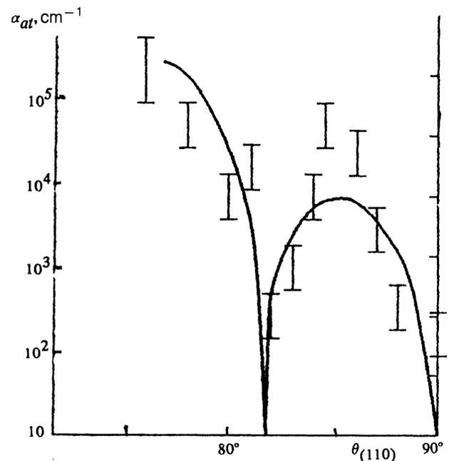
FIG. 3. Pseudosurface mode absorption as a function of the angle  $\theta_{(110)}$  for (111)-cut PbTe. The experimental error is indicated. The solid line was computed. The values of the material parameters for the curve were taken from Ref. 19.
