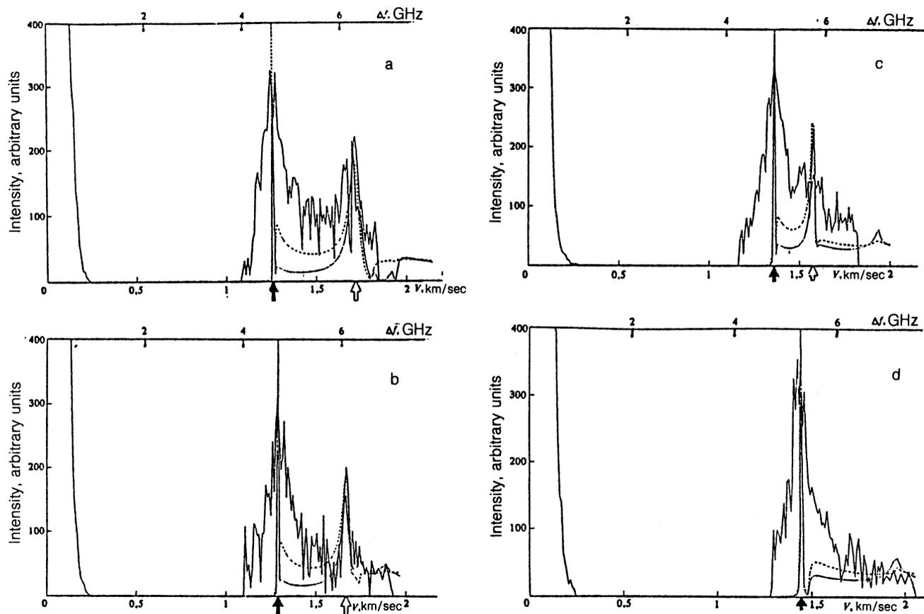
FIG. 4. Spectra of light scattered by a (111)-cut PbTe crystal for  $\theta_{(111)}=0^\circ$  (a),  $10^\circ$  (b),  $20^\circ$  (c), and  $30^\circ$  (d);  $\alpha=70^\circ$ . The arrows on the abscissa correspond to the GSW (dark-colored) and pseudosurface mode (light-colored) velocities. The computed SPDS spectrum of equilibrium surface excitations was calculated using the values given in Ref. [19] for the material parameters and is plotted in arbitrary units along the ordinate.
