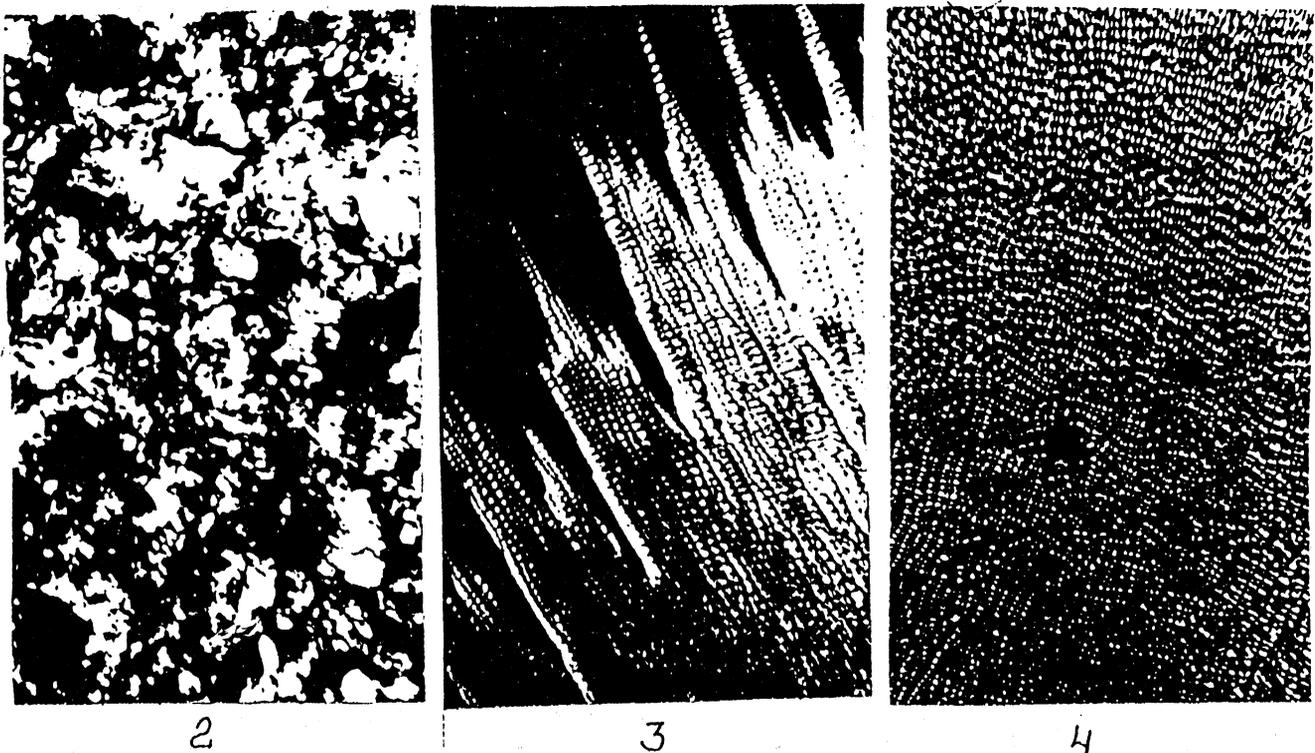
FIG. 2. Fragments of rings frozen in a crystal. 2—Polygonal texture; 3—outer edge of striated ring; 4—grid. (The photographs were taken through a Polam L-213 microscope.)
