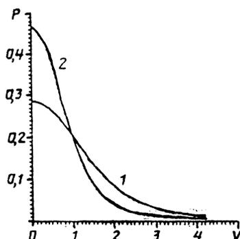
FIG. 3. The probability density of the potential for the dipole approximation. Curve 1 corresponds to the potential of a point dipole, and curve 2 to the potential of a dipole with a finite moment.
