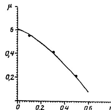
FIG. 4. The position of the Fermi level versus the degree of compensation (the points stand for the results of numerical modeling taken from Ref. 3).
