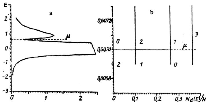
FIG. 5. The density of donor states in the limit of  $K \rightarrow 0$ : (a) the general shape of the  $N_d(E)/K$  vs  $E$  dependence (the maximum at zero is proportional to  $K^{-1/3}$  and is cut off in the figure); (b)  $N_d(E)/K$  near the Fermi level (0, 1, and 2 correspond to densities created by 0-, 1-, and 2-complexes and 3 corresponds to the total density  $N_d(E)/K$ ).
