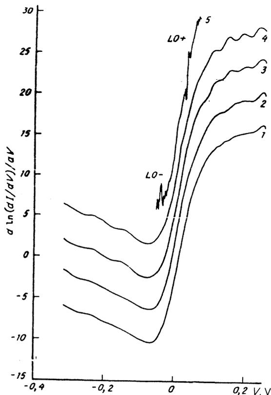
FIG. 4. Evolution of oscillations in time at  $p = 0$ : 1—before illumination; 2—9 min after illumination; 3—19 min after illumination; 4—35 min after illumination; 5—phonon singularities shown for the sake of comparison and recorded at  $T = 4.2$  K ( $LO^+$  represents characteristic singularities of the tunnel spectrum at energies equal to the energy of a longitudinal optical phonon in GaAs).
