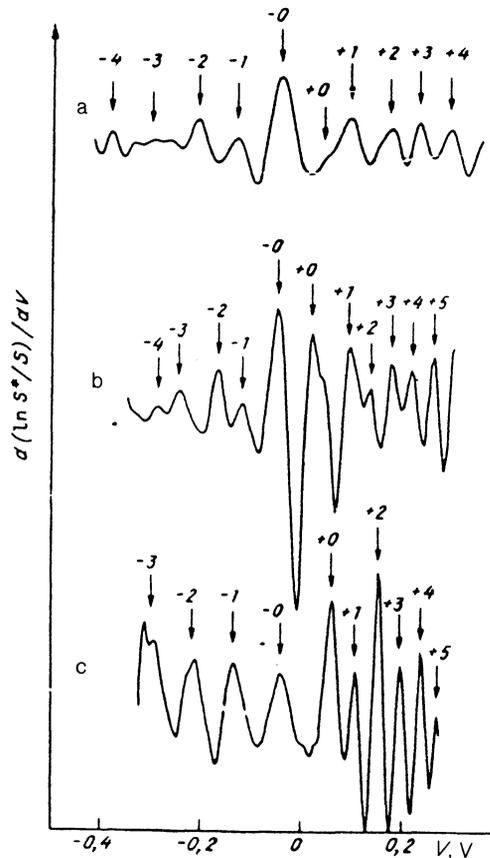
FIG. 5. Oscillation peaks of the logarithmic derivative of the ratio of the conductances at different pressures: a— $p = 10$  kbar; b— $p = 7$  kbar; c— $p = 0$ .
