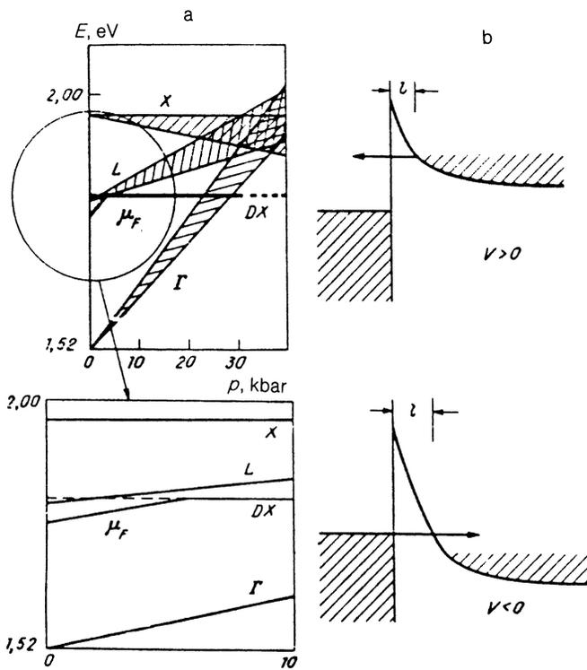
FIG. 6. a—Influence of the applied pressure on the structure of the conduction band of GaAs and the position of the Fermi level of electrons in a sample with  $N_d = 1.6 \times 10^{19} \text{ cm}^{-3}$ . b—Model of a Schottky barrier used in calculations of the screening length  $l$ .
