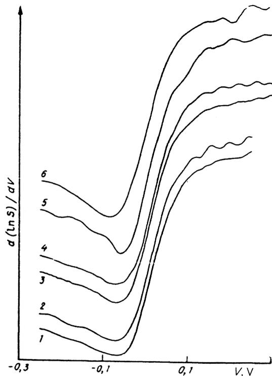
FIG. 3. Influence of illumination on the logarithmic derivative of the conductance at different pressures: 1,2— $p = 0$ ; 3,4— $p = 7$  kbar; 5,6— $p = 10$  kbar; 1,3,5—before illumination; 2,4,6—after illumination.
