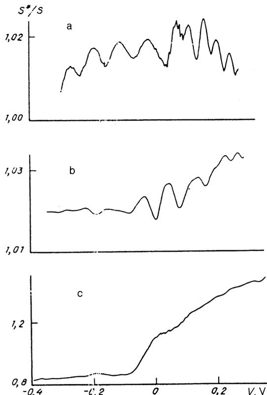
FIG. 1. Ratio of the tunnel conductance of an  $n$ -GaAs(Te)/Au junction after illumination ( $S^*$ ) to the dark conductance ( $S$ ), plotted as a function of the bias voltage  $V$  and recorded at different pressures: a— $p = 0$ ; b— $p = 7 \text{ kbar}$ ; c— $p = 10 \text{ kbar}$ .
