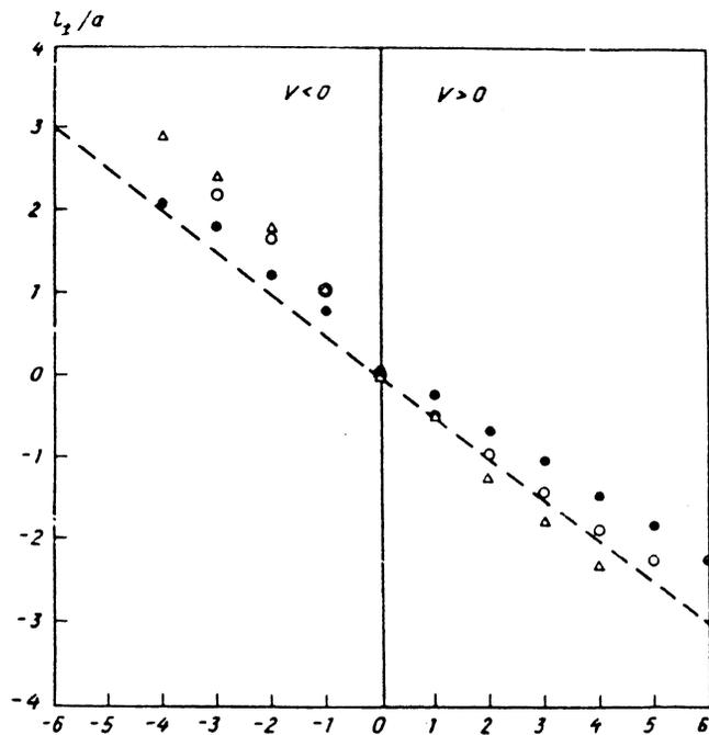
FIG. 7. Correlation of the oscillations with the position of the turning point for electrons at the Fermi of a semiconductor ( $V > 0$ ) or a metal ( $V < 0$ ;  $\circ$ — $p = 0$ ;  $\bullet$ — $p = 7$  kbar;  $\Delta$ — $p = 10$  kbar; the dashed line corresponds to the slope  $-1/2$ ). The abscissa gives the serial numbers of the peaks corresponding to those used in Fig. 5.
