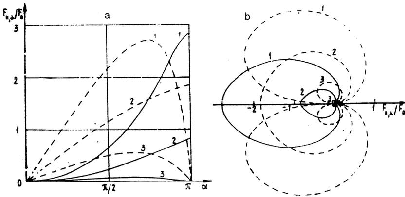
FIG. 5. The components of the radiative force as functions of the true angle  $\alpha$  for different velocities of a monopole source in a baroclinic model (a: in Cartesian, b: in polar coordinates):  $W/V_R = 0.5$  (1), 1 (2), 2 (3) [ $F_0 = (\rho\Gamma_m^2/4\pi)(\beta/V_R)^{1/2}$ ].
