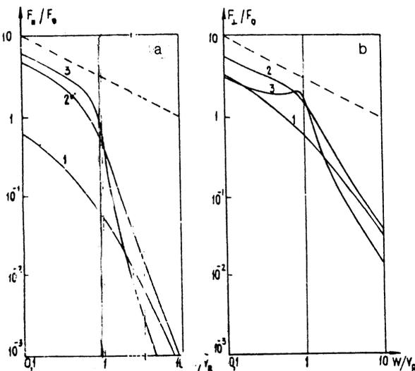
FIG. 6. The components of the radiative force (a— $F_{\parallel}$ , b— $F_{\perp}$ ) as functions of the velocity of a monopole source in a baroclinic model for three different angles:  $\alpha = \pi/4$  (1),  $3\pi/4$  (2),  $11\pi/12$  (3). The dashed line corresponds to a  $W^{-1/2}$  dependence [ $F_0 = (\rho\Gamma_m^2/4\pi)(\beta/V_R)^{1/2}$ ].
