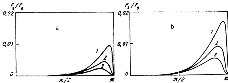
FIG. 7. The components of the radiative force (a— $F_{\parallel}$ , b— $F_{\perp}$ ) as functions of the true angle  $\alpha$  for different velocities of a dipole source in a baroclinic model:  $W/V_R = 1.01$  (1), 1.05 (2), 1.1 (3) [ $F_0 = (\rho\Gamma_d^2/4\pi)(\beta/V_R)^{3/2}$ ].
