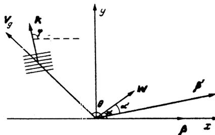
FIG. 1. A wave packet emitted by a moving source propagates with a group velocity  $v_g$  at an angle  $\theta$  to the  $x$ -axis, whereas the phase velocity of the waves is directed at an angle  $\varphi$  to the  $x$ -axis. The meaning of the vectors  $\beta$  and  $\beta'$  is explained in Sec. 3 of the text.
