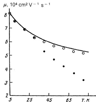
FIG. 4. The temperature curves representing the theoretical results (solid line) and experimental data<sup>10</sup> for the electron mobility in HgSe:Fe samples with  $N_{\text{Fe}} = 5.3 \cdot 10^{19} \text{ cm}^{-3}$ . The experimental values of  $\mu$  are depicted without the phonon contribution ( $\circ$ ) and with the phonon contribution ( $\bullet$ ).
