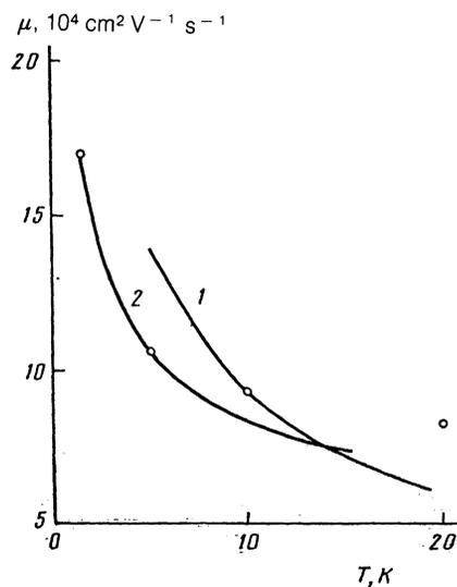
FIG. 5. The temperature curves representing the theoretical results (solid lines: curve 1,  $T_c = 5$  K; curve 2,  $T_c = 1$  K) and experimental data<sup>10</sup> for the electron mobility in HgSe:Fe samples with  $N_{Fe} = 1.8 \cdot 10^{19} \text{ cm}^{-3}$  (Refs. 10 and 13). In accordance with Ref. 11, the phonon-scattering contribution has been subtracted from the experimental values of  $\mu$ .
