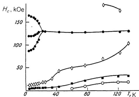
FIG. 1. Temperature curves for the fields  $H_c$  corresponding to the peaks in the absorption of microwave radiation in a  $\text{Ho}_{0.4}\text{Y}_{2.8}\text{Fe}_5\text{O}_{12}$  single crystal at  $\mathbf{H}||[111]$  and obtained at a probing frequency of 40.5 GHz. Different labels stand for different absorption lines.
