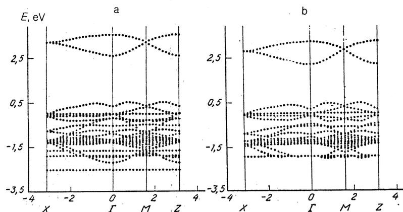
FIG. 1. Electron band structure of  $\text{La}_2\text{CuO}_4$  (a) and  $\text{Nd}_2\text{CuO}_4$  (b) (only the upper part of the valence band is shown).
