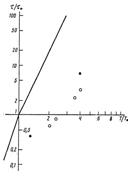
FIG. 6. Temperature dependence of the plasma heating rate under conditions corresponding to the anomalous skin effect. Solid line—Result of a self-similar solution under the assumption of a classical thermal conductivity, in accordance with (3) and (4); filled points—results of kinetic calculations with  $\alpha = 0.5$ ; open circles—the same, with  $\alpha = 0.25$ .
