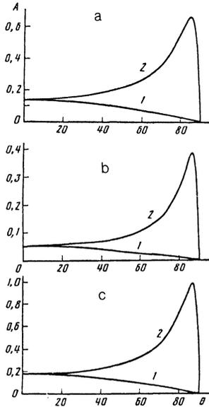
FIG. 9. Angular distribution of the absorption coefficient for (1) *s*-polarized and (2) *p*-polarized electromagnetic waves under conditions corresponding to the anomalous skin effect, with  $n_e/n_c = 100$  and  $v_{iz}/c = 0.1$ . a—The value of the anisotropy parameter is  $(\omega_p l_s/c)^2 \Delta = 0$ ; b— $-2$ ; c— $-5$ .
