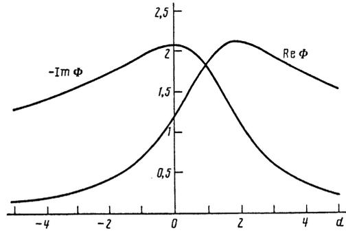
FIG. 8. Real and imaginary parts of the impedance versus the degree of anisotropy of the distribution function according to (20).
