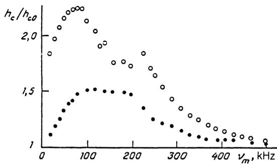
FIG. 2. Effect of modulation on the pumping threshold in the region of low hardness:  $h_{c10}/h_{c20} = 2.16$ ;  $\nu_p = 779.37$  MHz,  $T = 4.2$  K,  $H = 0.725$  kOe,  $H_m = 2.8$  Oe;  $\circ - h_{c2}$ ,  $\bullet - h_{c1}$ .
