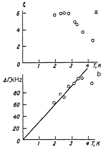
FIG. 6. a) Hardness parameter  $\xi = h_{c1}/h_{c2} - 1$  as a function of the temperature at the peak of the frequency dependence of  $\Delta\Gamma$  at  $H = 670$  Oe; b) temperature dependence of the turning-off part of the relaxation  $\Delta\Gamma$ ;  $H = 670$  Oe,  $\nu_p = 780$  MHz.
