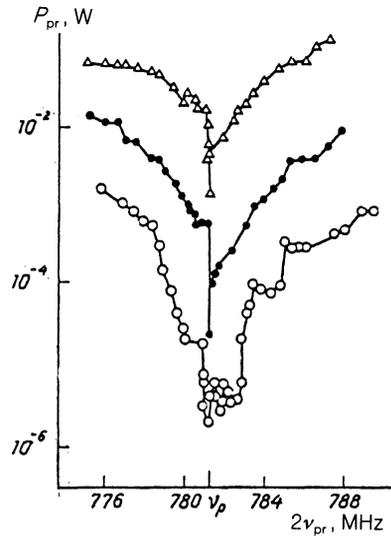
FIG. 9. Probe-pump power necessary for exciting magnons with frequency  $\nu_k = \nu_p/2 = 390.35$  MHz as a function of the probe-pump frequency for different main-pump amplitudes  $h$ :  $h/h_{c1} = 0.4$  ( $\Delta$ ),  $0.44$  ( $\bullet$ ),  $0.88$  ( $\circ$ ).  $T = 1.5$  K,  $H = 1120$  Oe.
