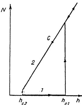
FIG. 10. Number of parametric magnons as a function of the microwave pump amplitude under conditions of hard excitation (schematically).
