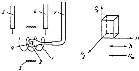
FIG. 1. Schematic diagram of the absorbing cell and the direction of the magnetic fields relative to the  $C_6$  axis of the crystal: 1) spiral resonator, 2) loop, 3) modulation coil, 4) sample, 5, 6, 7) coaxial waveguides from the pump generator, the receiving channel, and the probe-pump generator, respectively.
