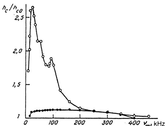
FIG. 3. Effect of modulation on the pumping thresholds in the region of high hardness:  $h_{c10}/h_{c20} = 5.65$ ;  $\nu_p = 778.7$  MHz,  $T = 1.76$  K,  $H = 1.08$  kOe,  $H_m = 1.96$  Oe;  $\circ - h_{c2}$ ,  $\bullet - h_{c1}$ .
