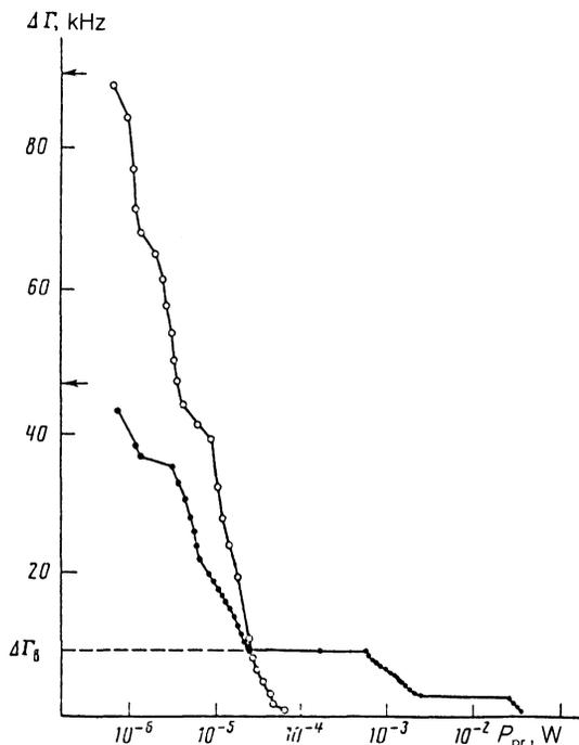
FIG. 8. Turning-off part of the relaxation as a function of the probe pump power with frequency  $\nu_{pr} = \nu_p/2 = 391.00$  MHz;  $\circ$ — $T = 4.2$  K,  $H = 750$  Oe;  $\bullet$ — $T = 1.5$  K,  $H = 1120$  Oe. The arrows mark the values of  $\Delta\Gamma$  for  $P_{pr} = 0$ .
