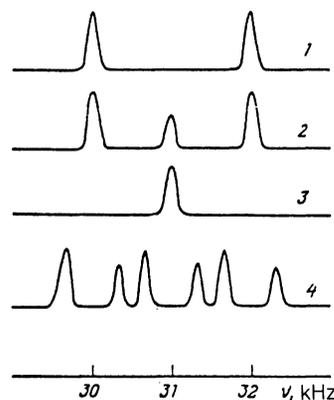
FIG. 4. Spectrum of the modulation response of the system of NSWs near the frequency  $\omega_m/2$  in the presence of two modulating fields with close frequencies:  $\omega_{m1} = 2\pi \cdot 60$  kHz and  $\omega_{m2} = 2\pi \cdot 64$  kHz. The spectra 1-4 correspond to different modulation amplitudes; the modulation increases from the first to the fourth spectrum.  $T = 1.82$  K,  $H = 1$  kOe,  $\omega_p = 2\pi \cdot 779.2$  MHz,  $H_{m1} \approx H_{m2}$ .
