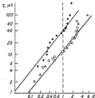
FIG. 12. Data from Fig. 11 in the  $\tau(X)$  coordinates, where  $X = -\ln \{ 1 - (h - h_{c2})^{1/2} / (h_{c1} - h_{c2})^{1/2} \}$ .  $\tau = T_1$  for  $X = 1$ .
