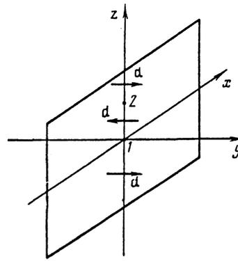
FIG. 2. Domain wall in the  $xz$  plane. The Bloch line runs along the  $z$  axis; 1 and 2 are the positions of two Bloch points;  $d$  is the orientation of a dipole moment on the Bloch line.
