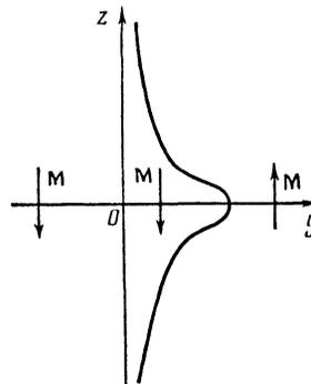
FIG. 3. Domain wall in the  $xz$  plane. The Bloch line is along the  $z$  axis; the Bloch point is the origin of coordinates; the domain wall displacement  $q(x, z)$  is along the  $y$  axis [ $q(-x, z) = -q(x, z)$ ].
