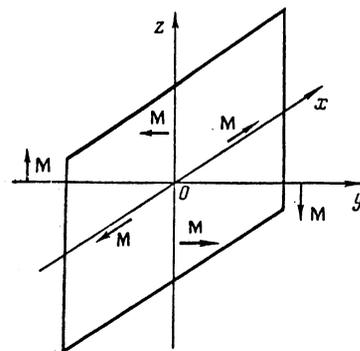
FIG. 1. Domain wall in the  $xz$  plane. The Bloch line runs along the  $z$  axis; the Bloch point is the origin of coordinates.
