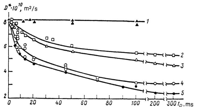
FIG. 2. Average self-diffusion coefficient  $D^*$  as a function of the diffusion time  $t_D$  for pure tridecane (curves 1), specimen No. 6 (2), No. 5 (3), No. 4 (4), and No. 3 (5).
