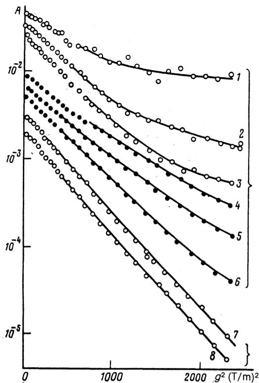
FIG. 1. Diffusive-damping curves for specimens Nos. 1 (curves 1), No. 2 (2), and No. 3 (3) with  $t_D = 6$  ms; specimen No. 4 with  $t_D = 310$  ms (4), 62 ms (5), and 6 ms (6) and specimen No. 6 with  $t_D = 310$  ms (7) and 13 ms (8). The measurement temperature was equal to 30 °C.
