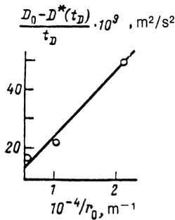
FIG. 4. Parameter  $(D_0 - D^*(t_D))/t_D$  as a function of the inverse radius of the sand grains in specimens Nos. 4, 5, and 6.
