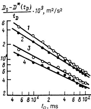
FIG. 3. Parameter  $(D_0 - D^*(t_D))/t_D$  as a function of the diffusion time  $t_D$  for specimens No. 3 (curve 1), No. 4 (2), No. 5 (3), and No. 6 (4). The measurement temperature is equal to 30 °C.
