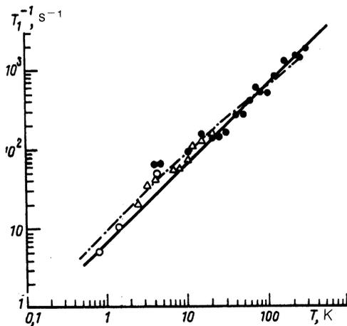
FIG. 4. Temperature dependence of the spin-lattice relaxation rate of  $^{63}\text{Cu}$  nuclei in  $\text{Pr}_{2-x}\text{Ce}_x\text{CuO}_{4-y}$ :  $\bullet$  (70 MHz),  $\Delta$  (12 MHz)—data from Ref. 12, (22.5 MHz)—our measurements; the straight line is Korringa's law (1); the dot-dashed line is  $T_1^{-1} = T_1^{-1} + 4.6T$  (see text).
