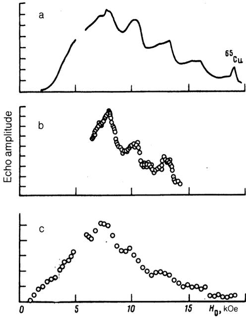
FIG. 6. NMR spectra of  $^{141}\text{Pr}$  in oriented PrCeCuO powder at a frequency of 23 MHz in a field  $H_0 \parallel c$ : a)  $T = 1.6$  K,  $t_{\pi/2} = 1.1$   $\mu\text{s}$ ,  $\tau = 7$   $\mu\text{s}$ ; b)  $T = 1.05$  K,  $t_{\pi/2} = 1$   $\mu\text{s}$ ,  $\tau = 7$   $\mu\text{s}$ ; c)  $T = 0.10$  K,  $t_{\pi/2} = 0.9$   $\mu\text{s}$ , and  $\tau = 10$   $\mu\text{s}$ .
