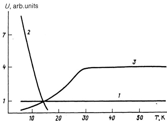
FIG. 7. Computed temperature dependence of the amplitudes  $U$  of nonlinear generation of longitudinal ultrasound in Zn at the frequency of the electromagnetic wave 9.5 MHz in an alternating magnetic field of 35 Oe by induction (curve 1), deformation (curve 2), and thermoelastic (Fig. 3) conversion mechanisms.
