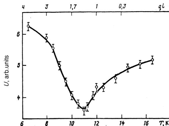
FIG. 5. Temperature dependence of the amplitude  $U$  of ultrasound generated in Zn by the nonlinear mechanism at the frequency of the electromagnetic wave 5 MHz. The intensity of the rf magnetic field is equal to 35 Oe.
