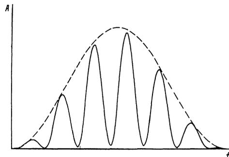
FIG. 2. Amplitude-frequency characteristics of a composite resonator consisting of a piezoelectric transducer and the specimen. The dashed line is the amplitude-frequency characteristic of the piezoelectric transducer itself.
