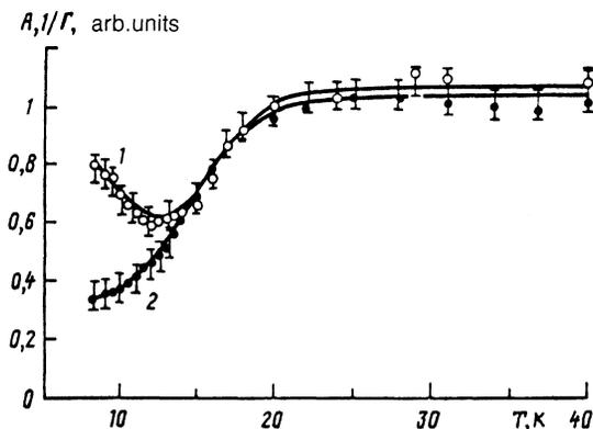
FIG. 3. Temperature dependences of the amplitude  $A$  of the acoustic resonance in the specimen (curve 1) and the inverse attenuation  $1/\Gamma$  (curve 2) at an ultrasonic frequency of 19 MHz. The curves are normalized to the values of  $A$  and  $1/\Gamma$  at high temperatures.
