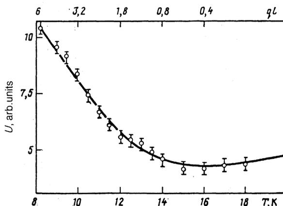
FIG. 6. Temperature dependence of the amplitude  $U$  of nonlinear generation of longitudinal ultrasound in Zn at the frequency of the electromagnetic wave 9.5 MHz. The intensity of the rf magnetic field is equal to 35 Oe.
