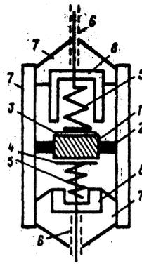
FIG. 1. Layout of the measuring chamber: 1) specimen, 2) indium screen, 3) piezoelectric transducer, 4) spiral induction coil, 5) springs, 6) coaxial cables, 7) box, 8) insulator.
