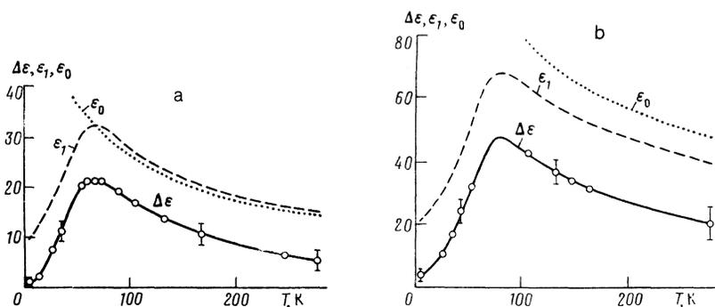
FIG. 4. Temperature dependences of dielectric contribution Δε of the soft mode of the dielectric constant ε<sub>1</sub> at the frequency ~ 1 cm<sup>-1</sup> and of the static ε<sub>0</sub> (Refs. 17, 18) in polarizations E∥c (a) and E⊥c (b).
