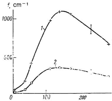
FIG. 5. Temperature dependences of soft-mode oscillator strengths 1— $E \perp c$ , 2— $E \parallel c$ .
