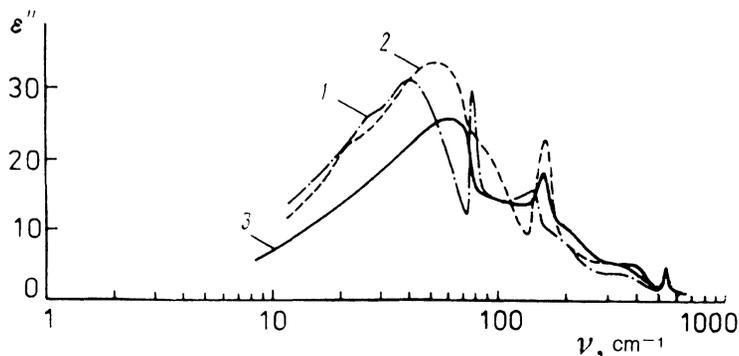
FIG. 2. Comparison of  $\epsilon''(\nu)$  spectra, for  $E\perp c$ , of pure RDP (1) and ADP (2) crystals<sup>13,14</sup> and of mixed RADP (3) (see Fig. 1b).
