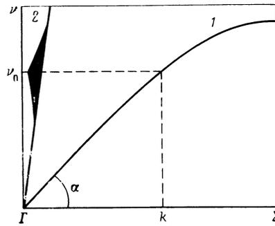
FIG. 6. Scheme of interaction between cluster-structure oscillations with wave vector  $k$  and acoustic oscillations; and  $\Sigma$  are the center and boundary of the Brillouin zone; 1—acoustic mode,  $\alpha$ —inclination angle (speed of sound); 1—IR-active mode.
