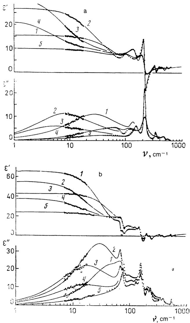
FIG. 1. Dielectric spectra  $\epsilon'(\nu)$  and  $\epsilon''(\nu)$  of RADP dipole glass in orientations  $E||c$  (a) and  $E\perp c$  (b) at temperatures ( $T$ , K) 1—275, 2—108, 3—53, 4—35, 5—5. Points in the region  $\nu \sim 10 \text{ cm}^{-1}$ —submillimeter backward wave tube spectroscopy data, above  $40 \text{ cm}^{-1}$ —calculated using the Kramers–Kronig equations from IR reflection spectra. Solid lines—model of independent oscillators.
