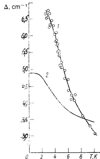
FIG. 3. The temperature dependence of the splitting between the lower doublets of the ground state of the  $\text{Ce}^{3+}$  ion in Ce ETS. 1) The values of  $\Delta$  determined experimentally in the present work; 2) the curve constructed from the data of Ref. 5.
