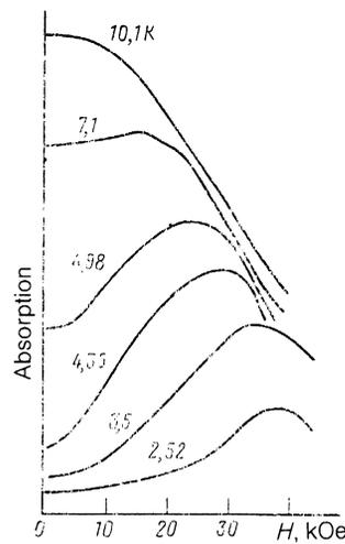
FIG. 2. The form of the spectrum of the  $\text{Ce}^{3+}$  ion in Ce ETS at different temperatures.
