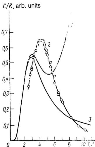
FIG. 4. The temperature dependence of the molar heat capacity of Ce ETS. 1) The curve experimentally obtained in Ref. 1; 2) the curve calculated from the dependence  $\Delta(T)$  determined experimentally in the present work; 3) the temperature dependence of the heat capacity of Ce ETS in the absence of spin-lattice coupling (Schottky heat capacity<sup>1</sup>).
