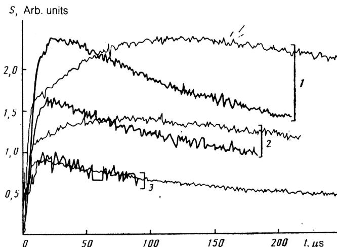
FIG. 3. Signals representing the deviation from a phonon equilibrium detected by a bolometer in samples of  $Y_{2.8}Er_{0.2}Al_5O_{12}$  and  $Y_{2.8}Lu_{0.2}Al_5O_{12}$  (the brighter line) with  $L = 0.68$  cm for various sample temperatures: 1— $T = 3.83$ , 2— $3.43$ , 3— $2.91$  K.  $P_H = 10^{-2}$  W/mm<sup>2</sup>,  $l_H/L = 1$ .
