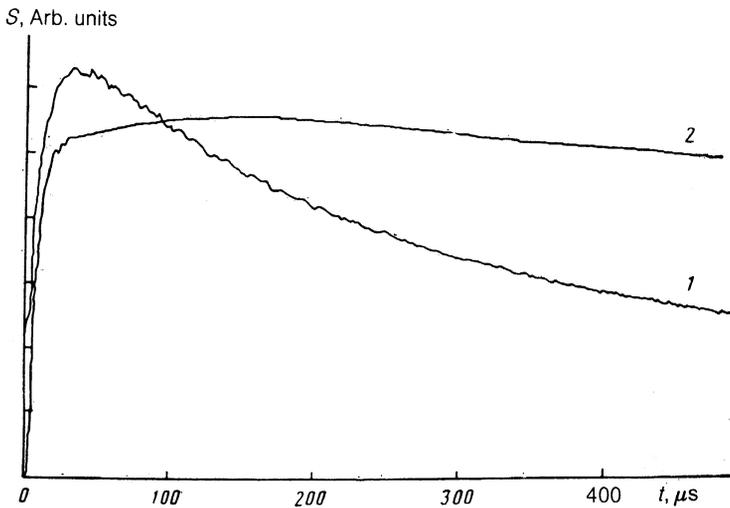
FIG. 9. Signals representing the deviation from a phonon equilibrium in certain samples. 1—CNGG; 2—(10% Er):CNGG.  $L_{1,2} = 0.5$  cm,  $T = 3.4$  K,  $P_H < W/\text{mm}^2$ .
