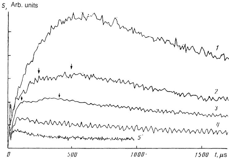
FIG. 5. Signals representing the deviation from a phonon equilibrium detected by a bolometer in a sample of  $Y_{2.4}Er_{0.6}Al_5O_{12}$ ;  $L = 0.68$  cm. 1— $T = 3.78$ ; 2—3.41; 3—3.18; 4—2.99; 5—2.73 K.
