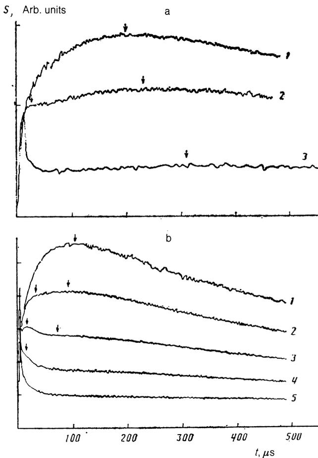
FIG. 4. Signals representing the deviation from a phonon equilibrium detected by a bolometer in a sample of  $Y_2Er_1Al_5O_{12}$ . a:  $L = 0.14$  cm. 1— $T = 3.44$ ; 2—3.08; 3—2.71 K. b:  $L = 0.065$  cm. 1— $T = 3.83$ ; 2—3.5; 3—3.21; 4—2.99; 5—2.69 K.  $P_H = 0.1$  W/mm<sup>2</sup>.
