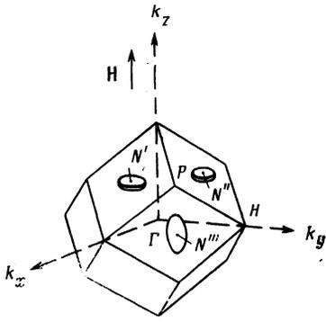
FIG. 3. Positions of the hole  $N$  ellipsoids with respect to the center of the Brillouin zone,  $\Gamma$ . The heavy lines on the ellipsoids centered at  $N'$  and  $N''$  show the cross sections which cause the quantum oscillations in the ultrasonic parameters in tungsten for the given field configuration.
