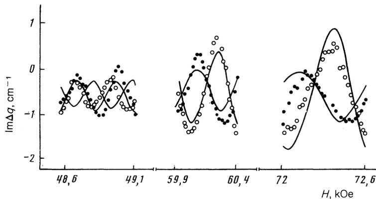
FIG. 5. Magnetic-field dependence of the imaginary part of the wave vector of the ultrasound. ●, ○—experimental data for the  $-$  polarization and the  $+$  polarization, respectively; solid lines—theoretical predictions from expression (13).
