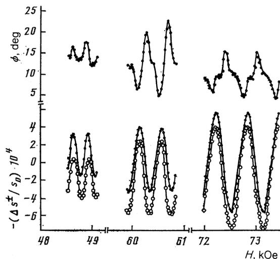
FIG. 2. Magnetic-field dependence of the velocities of circularly polarized waves and of the angle through which the polarization plane of the ultrasound is rotated. ● — polarization; ○ — + polarization.
