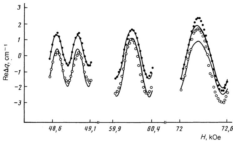
FIG. 6. Magnetic-field dependence of the real part of the wave vector of ultrasound. ●, ○—Experimental data for the — polarization and the + polarization, respectively; solid lines—theoretical predictions from (12).
