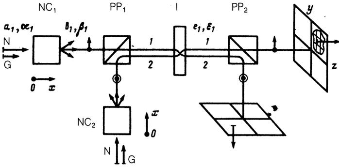
FIG. 1. The optical scheme used for interference mixing of "squeezed" orthogonally polarized light beams: NC are nonlinear crystals,  $I$  is an interference device, and  $PP_1$  and  $PP_2$  are polarization prisms, which combine and separate in space light waves with distinguished polarizations. A dense array of efficient photon counters is shown, in part, in one of the detection planes.
