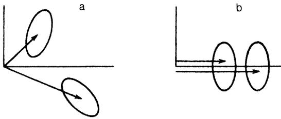
FIG. 2. Matching of the phases of the reference and "squeezed" waves arriving from two inputs on one of the detectors of the optical image: a) general case and b) fluctuations of the intensity are suppressed in proportion to squeezing.
