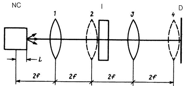
FIG. 3. Compensation of diffraction in the output layer of the nonlinear crystal and under conditions of free propagation with the help of focusing.
