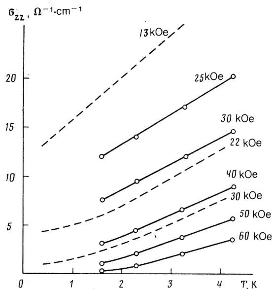
FIG. 5. The temperature dependence  $\sigma_{zz}(T)$  for  $n$ -InSb with  $\mathbf{j}||z$  and  $\mathbf{H}||z$ . The solid lines are our data for sample No. 2 with  $n = 3.3 \cdot 10^{15} \text{ cm}^{-3}$  and the dashed lines are the data of Ref. 8 for  $n$ -InSb with  $n = 2.2 \cdot 10^{15} \text{ cm}^{-3}$ .
