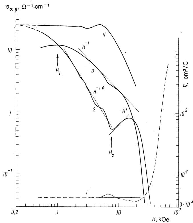
FIG. 1. The conductivities  $\sigma_{\alpha\beta}$  and the Hall coefficient  $R$  as a function of the magnetic field  $H$  for sample No. 1  $n$ -InSb ( $n = 1.5 \cdot 10^{15} \text{ cm}^{-3}$ ). Curve 1— $R(H)$ ; 2— $\sigma_{xx}(H)$ ; 3— $\sigma_{xy}(H)$  with  $\mathbf{j}||x$  and  $\mathbf{H}||z$ ; 4— $\sigma_{zz}(H)$  with  $\mathbf{j}||z$  and  $\mathbf{H}||z$ .
