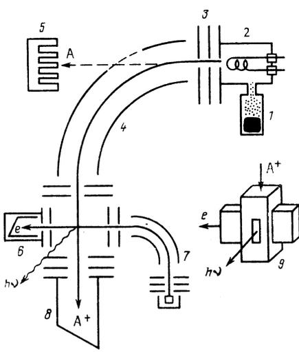
FIG. 1. Schematic diagram of the apparatus: 1) reservoir with the working substance; 2) ionization chamber; 3) ion-optical system; 4) electrostatic ion selector; 5) traps for atoms; 6) electron collector; 7) source of electrons; 8) ion collector; 9) intersecting beam configuration ( $e$  denotes electrons,  $A^+$  denotes ions, and  $h\nu$  is the emitted radiation).
