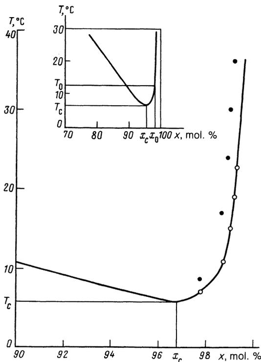
FIG. 1. Phase diagram of a solution of TMP in water; the solid curve is the binodal from Ref. 4;  $\circ$  denotes the series of experimental points  $T_1$ ,  $\bullet$  are the corresponding spinodal points  $T_2$ . In the inset we show the general form of the binodal.
