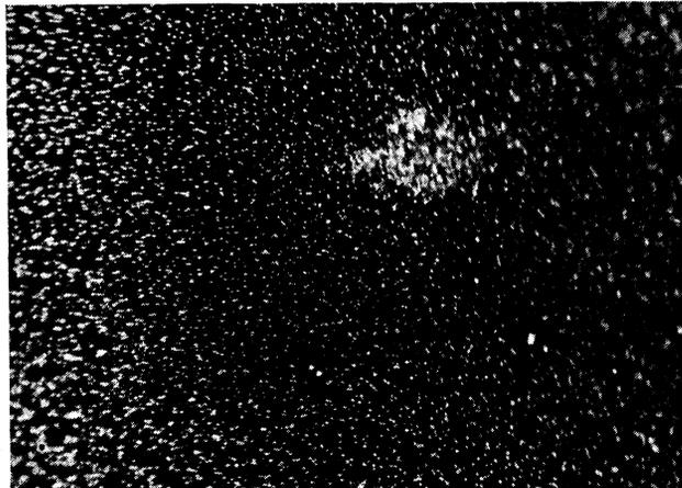
FIG. 4. Formation of a dark spot with an increased quantity of microdroplets of the LF as a result of a laser shot.
