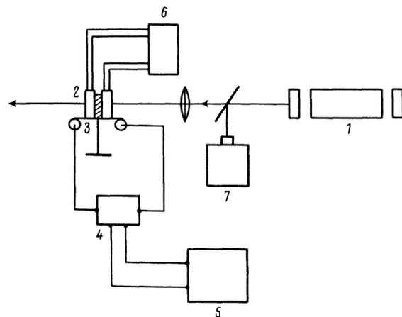
FIG. 2. Schematic experimental setup: 1—YAG:Nd<sup>3+</sup> laser, 2—cuvette with solution, 3—2-coordinate stage, 4—CAMAC module, 5—IBM-PC-XT, 6—thermostat, 7—IMO-2H energy meter for measuring the laser radiation.
