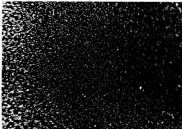
FIG. 3. General form of microdroplets of the LF in an HF solution for  $T_0 = T_b(x_0)$ .
