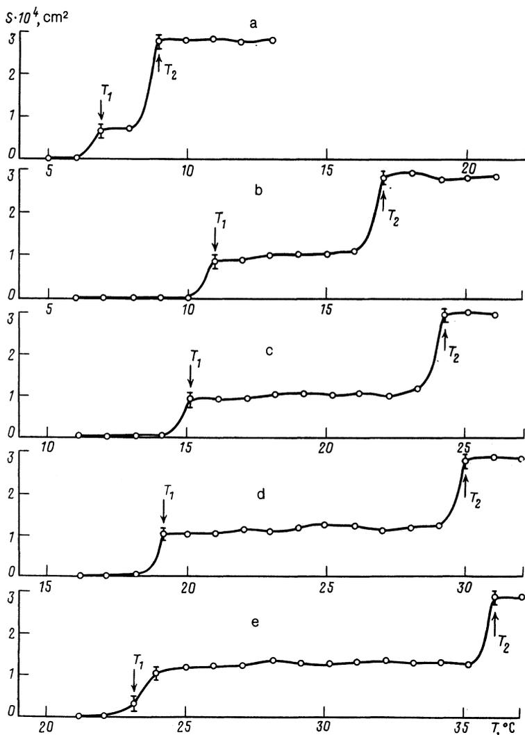
FIG. 5. Temperature dependence of the area  $S$  produced by laser action: a)  $T_0 = 7^\circ\text{C}$ ,  $x_0 = 98$  mole %; b)  $T_0 = 11^\circ\text{C}$ ,  $x_0 = 99$  mole %; c)  $T_0 = 15^\circ\text{C}$ ,  $x_0 = 99.15$  mole %; d)  $T_0 = 19^\circ\text{C}$ ,  $x_0 = 99.3$  mole %; e)  $T_0 = 23^\circ\text{C}$ ,  $x_0 = 99.5$  mole %.
