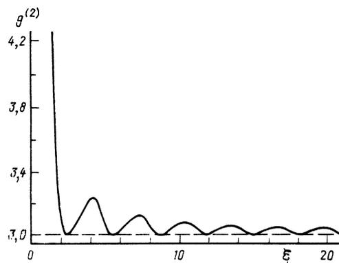
FIG. 5. Dependence, on the parameter  $\xi$ , of the normalized correlation function of the intensity of light of the mode  $\omega_0$  at the resonator exit.
