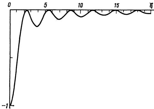
FIG. 2. Dependence of the ratio  $\text{Re } \alpha_0/\sigma$  of the nonlinear absorption coefficient to the conventional absorption coefficient on the parameter  $\xi$ .
