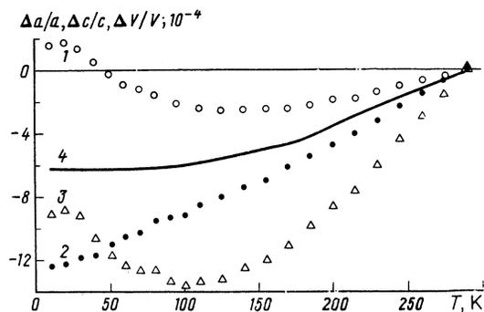
FIG. 4. Temperature dependences of the relative unit cell parameters  $\Delta a/a$  [curve 1,  $a(290 \text{ K}) = 6.9428 \text{ \AA}$ ],  $\Delta c/c$  [curve 2,  $c(290 \text{ K}) = 6.0712 \text{ \AA}$ ], of the volume  $\Delta V/V$  (curve 3) of the tetragonal unit cell of  $\text{TbPO}_4$ , and of the relative value of the parameter  $\Delta a/a$  of  $\text{YPO}_4$  (curve 4).
