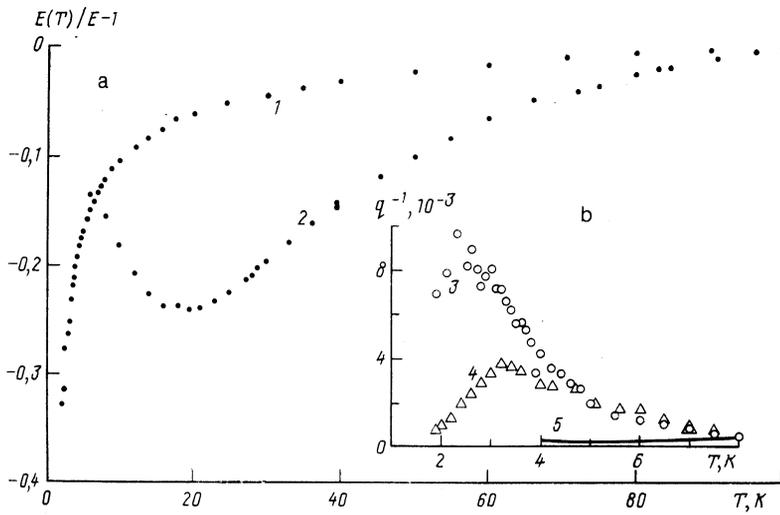
FIG. 1. Temperature dependences of the relative value of the Young modulus  $E(T)/E - 1$  (a) and of the internal friction  $q^{-1}$  (b) of polycrystalline samples of  $\text{TbPO}_4$  ( $H = 0$  for curves 1 and 3 and  $H = 30$  kOe for curve 4) and  $\text{TmPO}_4$  ( $H = 0$  for curves 2 and 5).
