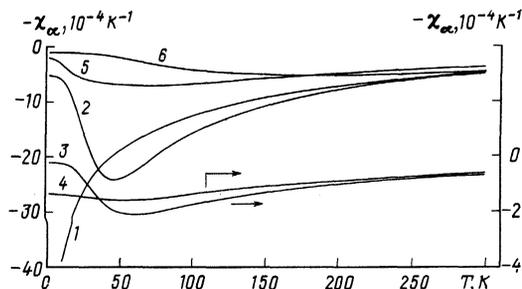
FIG. 8. Calculated temperature dependences of the deformation susceptibility  $\chi_\alpha$  of the following rare-earth phosphates: 1) TbPO<sub>4</sub>; 2) DyPO<sub>4</sub>; 3) HoPO<sub>4</sub>; 4) ErPO<sub>4</sub>; 5) TmPO<sub>4</sub>; 6) YbPO<sub>4</sub>.
