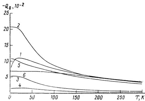
FIG. 7. Calculated temperature dependences of the quadrupole moment  $Q_0$  of the following rare-earth phosphates: 1)  $\text{TbPO}_4$ ; 2)  $\text{DyPO}_4$ ; 3)  $\text{HoPO}_4$ ; 4)  $\text{ErPO}_4$ ; 5)  $\text{TmPO}_4$ ; 6)  $\text{YbPO}_4$ .
