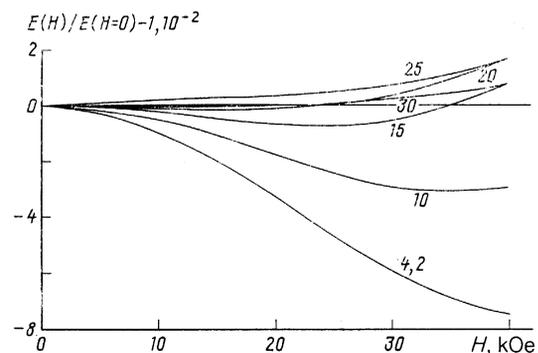
FIG. 2. Field dependences of the relative value of the Young modulus of a polycrystalline sample of  $\text{TmPO}_4$ , determined at low temperatures.
