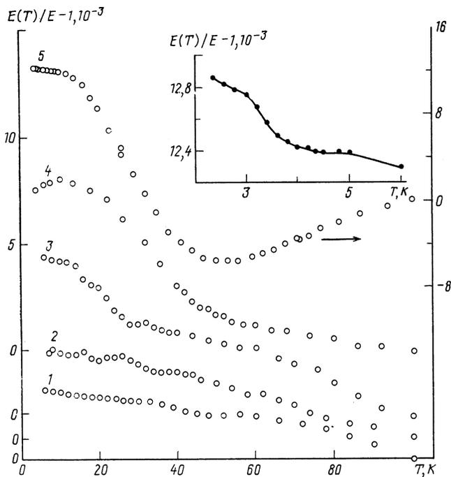
FIG. 3. Temperature dependences of the relative Young modulus of polycrystalline samples of  $\text{YPO}_4$  (1),  $\text{YbPO}_4$  (2),  $\text{ErPO}_4$  (3),  $\text{HoPO}_4$  (4), and  $\text{DyPO}_4$  (5). The inset shows the behavior of the Young modulus of  $\text{DyPO}_4$  at low temperatures.
