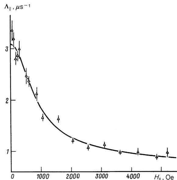
FIG. 1. Relaxation rate of the muon spin,  $\Lambda_{\parallel}$ , versus the longitudinal magnetic field  $H_{\parallel}$ . The solid line shows the theoretical  $\Lambda_{\parallel}^{\text{theo}}(H_{\parallel})$  dependence [see (13)].
