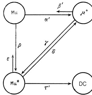
FIG. 3. Schematic diagram of the relaxation of the muon spin in silicon.  $Mu$ —normal muonium;  $Mu^*$ —anomalous muonium;  $\mu^+$ —free muon; DC—diamagnetic (chemical) compound.
