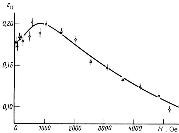
FIG. 2. The  $c_{\parallel}(H_{\parallel})$  dependence, i.e., the asymmetry coefficient of the angular distribution of positrons from the decay  $\mu^+ \rightarrow e^+$  versus the longitudinal field  $H_{\parallel}$ . The solid line is the theoretical  $c_{\parallel}^{\text{theo}}(H_{\parallel})$  dependence [see (12)].
