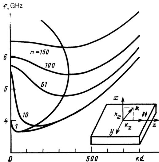
FIG. 4. Spectrum of backward internal magnetostatic waves for an YIG film  $20 \mu\text{m}$  thick for  $n = 1, 10, 61, 100, 150$ . Magnetic field  $H = 1300 \text{ Oe}$ . The double-valued trace corresponds to waves with group velocity  $v = 0$  that have the minimum threshold of local parallel pumping. Inset—coordinate system and direction  $\mathbf{H}$ ,  $\mathbf{k}$  for a tangentially magnetized film.
