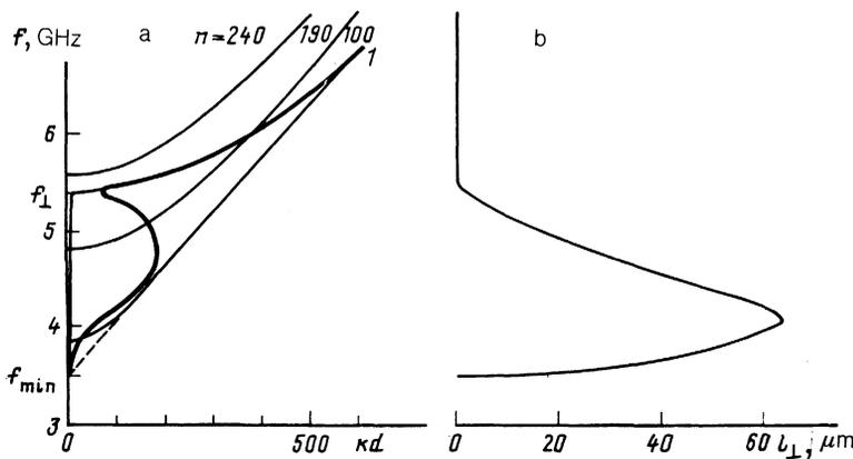
FIG. 3. a—Spectrum of primary internal magnetostatic waves for an YIG film  $20 \mu\text{m}$  thick for  $n = 1, 100, 190, 240$ . Constant field  $H = 3000$  Oe. Double-valued trace corresponds to waves having a minimum threshold of local parallel pumping. b—Path length of spin waves along the normal to the surface of the film for waves denoted by the double-valued trace in Fig. 3a.
