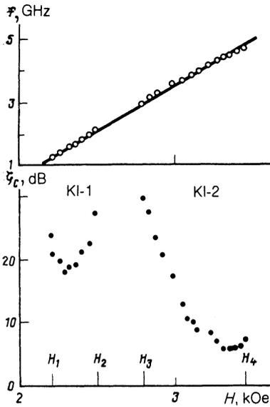
FIG. 1. Threshold supercriticality of KI  $\zeta_c$  (●) and frequency  $f$  of the emission arising at the threshold (○) as a function of constant magnetic field  $H$  for a perpendicularly magnetized YIG film  $20 \mu\text{m}$  thick. Straight line—frequency of the bottom of the SW spectrum;  $H_1$  and  $H_2$ ,  $H_3$  and  $H_4$ —boundaries of experimental regions within the confines of which KI is observed.
