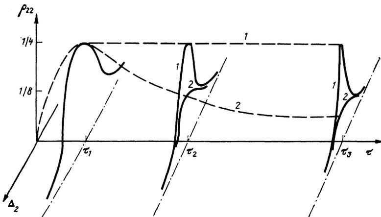
FIG. 5. Population of the upper level,  $\rho_{22}$ , as a function of the time  $\tau$  and of the deviation from resonance,  $\Delta_2$ . 1— $\alpha = 0$ ; 2— $\alpha \neq 0$ . Dashed lines)  $\Delta_2 = 0$ ; dot-dashed lines) sections at identical times  $\tau_1 \sim (8\pi g E^2 \mu^2)^{-1}$ ,  $\tau_1 < \tau_2 < g$ ,  $\tau_3 \gtrsim g$ .
