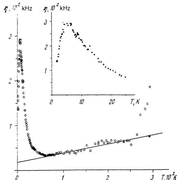
FIG. 6. Temperature dependence of phonon relaxation rate in specimen No. 2 for  $\omega_p/2\pi = 600$  MHz,  $H = 230$  Oe;  $\circ$ ) calculated according to Eq. (3),  $+$ ) measured by the modulation method. The straight line is a plot of the empirical formula for  $\eta_2$  (see text).
