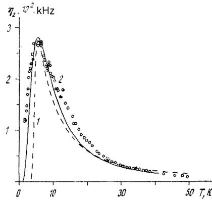
FIG. 8. Temperature dependence of the phonon relaxation parameter  $\eta_2 = \eta - \eta_1$  for  $\omega_p/2\pi = 600$  MHz,  $H = 230$  Oe. The dashed curve 1 is calculated from Eq. (8) with the impurity relaxation in the form of Eq. (6). The full curve 2 is calculated according to Eq. (8) with the impurity relaxation in the form of Eq. (9).
