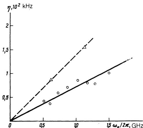
FIG. 5. Dependence of phonon relaxation rate on the pumping frequency for two specimens:  $\triangle$ ) specimen No. 1,  $\circ$ ) specimen No. 2;  $T = 77$  K,  $H = 330$  Oe.
