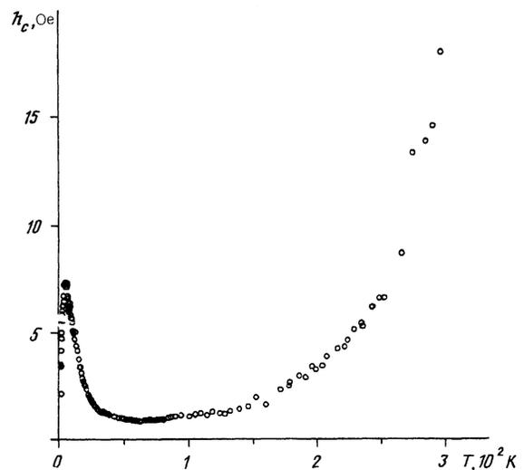
FIG. 3. Temperature dependence of the parallel pumping threshold;  $\omega_p/2\pi = 600$  MHz,  $H = 230$  Oe.
