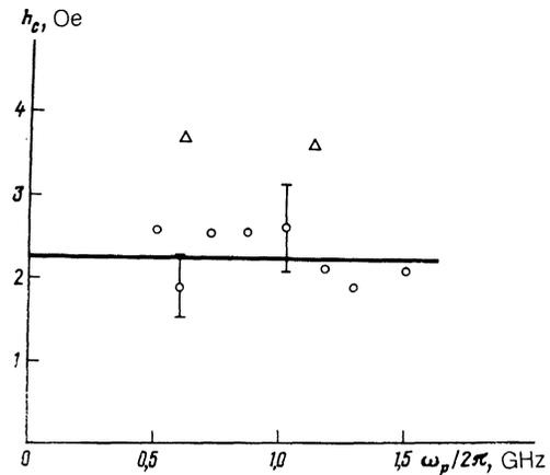
FIG. 2. Frequency dependence of the parallel pumping threshold for two specimens:  $\Delta$ ) specimen No. 1,  $\circ$ ) specimen No. 2;  $T = 77$  K,  $H = 330$  Oe.
