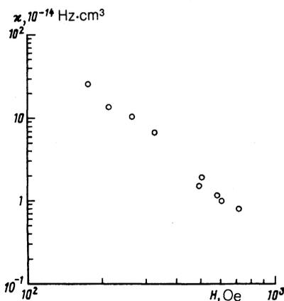
FIG. 13. The coefficient of nonlinear attenuation of phonons as a function of the magnitude of the steady magnetic field;  $T = 77$  K,  $\omega_p/2\pi = 1450$  MHz,  $\xi = 1.5$ .
