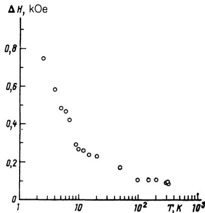
FIG. 9. Temperature dependence of the EPR linewidth of the paramagnetic impurity for  $\omega_p/2\pi = 9.45$  GHz.
