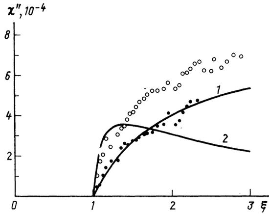
FIG. 11. Nonlinear magnetic susceptibility  $\chi''$  of phonons as a function of the excess of the pumping field amplitude above threshold  $\xi = h/h_c$ : (O)  $H = 266$  Oe; (●) 496 Oe;  $\omega_p/2\pi = 1450$  MHz,  $T = 77$  K. Curve 1—calculated according to Eq. (11). Curve 2—calculated according to Eq. (12).
