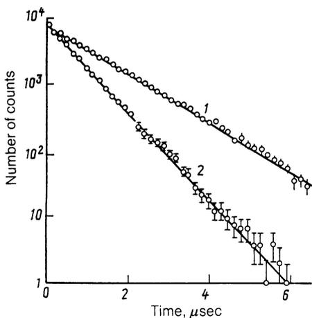
FIG. 3. Time distributions of the first detected neutrons from the  $dd$ -fusion reaction: 1—experiment with pure deuterium; 2—experiment with a  $\text{D}_2 + ^4\text{He}$  mixture ( $C_{\text{He}} = 0.31\%$ ); solid curves—result of fits.
