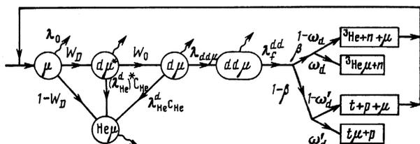
FIG. 1. Diagram of muon-atom and muon-molecule processes occurring in a  $\text{D}_2 + {}^4\text{He}$  mixture.
