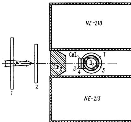
FIG. 2. Diagram of experimental apparatus for study of the transfer of muons from  $d\mu$  atoms to  ${}^4\text{He}$  nuclei.
