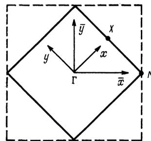
FIG. 1. Brillouin zones of an antiferromagnet (continuous line) and a normal metal (dashed line) with a square crystal lattice:  $\Gamma$ ,  $M$ , and  $X$  are the characteristic (high-symmetry) points.
