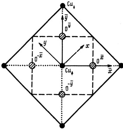
FIG. 2. Distribution of copper and oxygen atoms in an antiferromagnetic cell of  $\text{CuO}_2$ .
